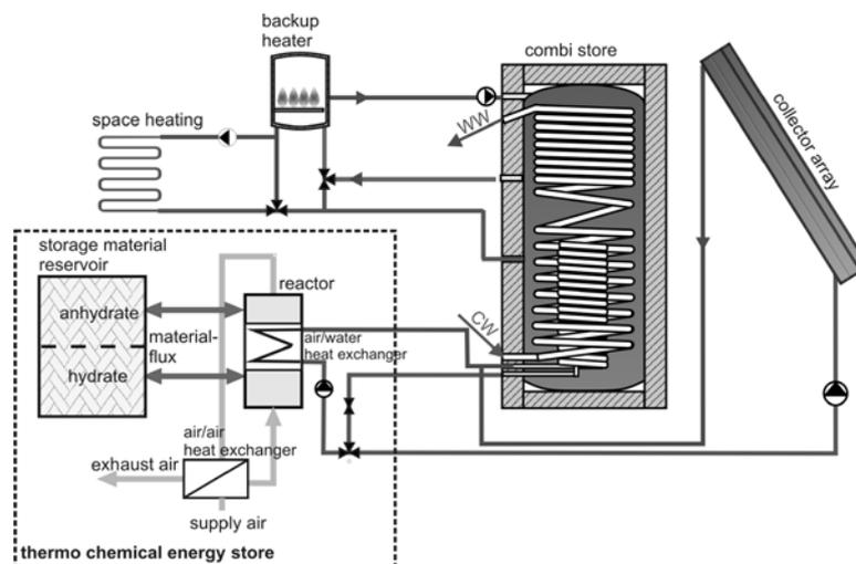
Figure 1: Schematic of a solar combisystem with thermo-chemical energy store.
