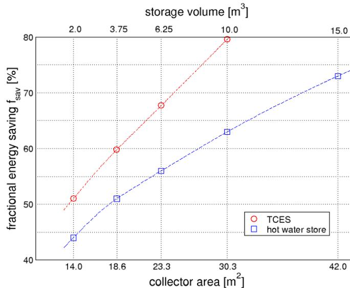
Figure 2: Fractional energy savings of a large solar combisystem with hot water store and a thermo-chemical energy store (TCES)
