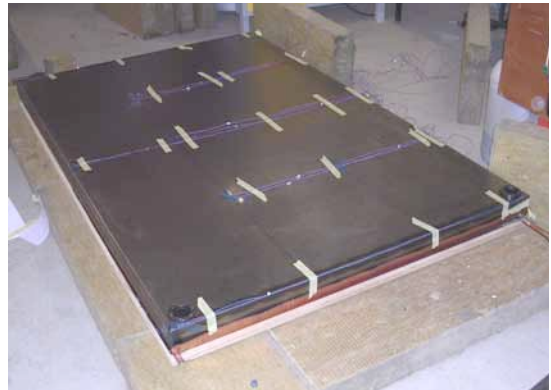
Figure 3. Seasonal heat storage module test at DTU in Denmark.
