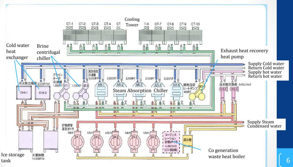
(※)In this plant we have adapted the electric and gas combined system. And load leveling has been achieved by ice storage system utilizing nighttime electric power and use of steam absorption chiller. Also waste heat from the cogeneration system (Natural gas) which is installed inside the JR central tower building is used.
