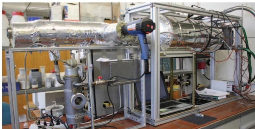
Figure 2. Photograph of the thermal adsorption storage (open system).
