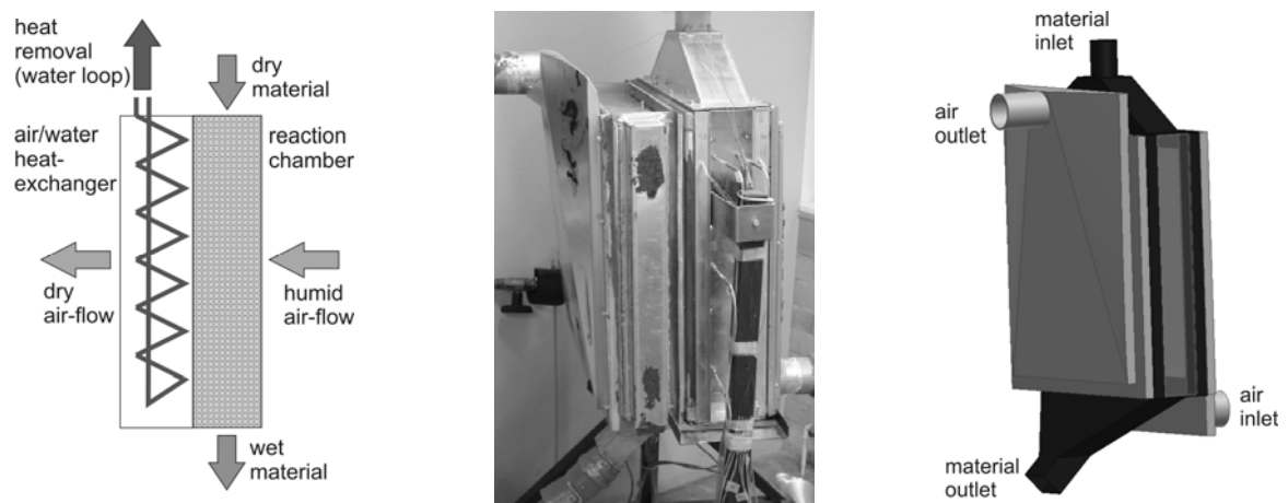
Figure 2: Cross-flow reactor concept in heating mode (left), test reactor in lab-scale (middle) and construction plan (right).
