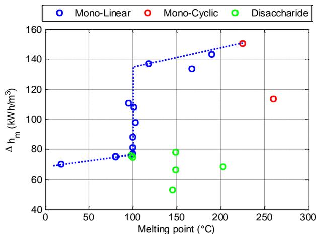
Enthalpy change by melting of polyols as a function of the melting point.
