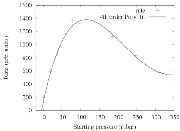
*Dehydration rate as a function of starting water vapor pressure. This curve shows the Topley-Smith effect.*
