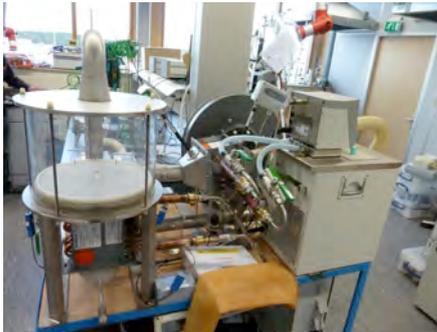
*ECN's bulk type open sorption prototype reactor.*
